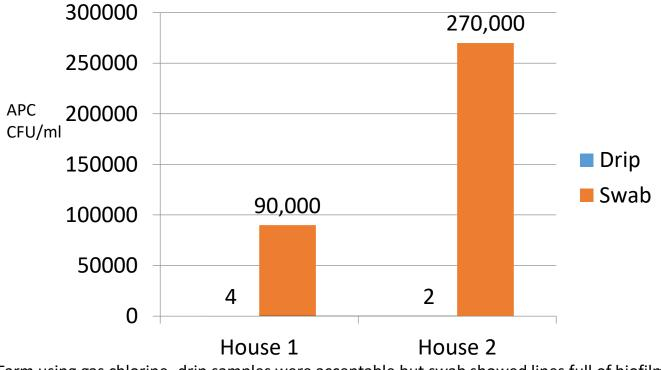
Farm using gas chlorine- drip samples were acceptable but swab showed lines full of biofilm
